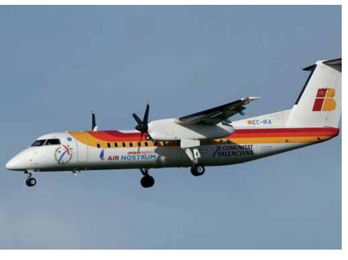
The three main Dash 8 variants have similar cruise speeds of 265-300 knots. The Q400 is faster at 360 knots.
