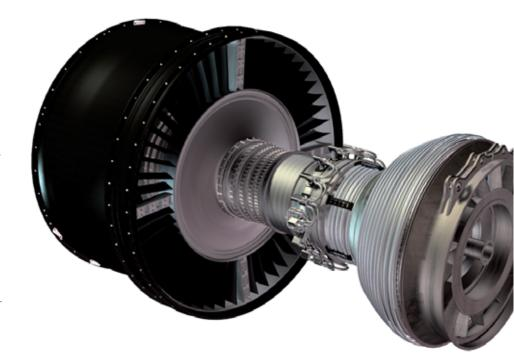
The small diameter of the LEAP-X's core engine is illustrated by this computer representation of the engine, and demonstrates how the engine's bypass ratio of 12:1 will be achieved.
