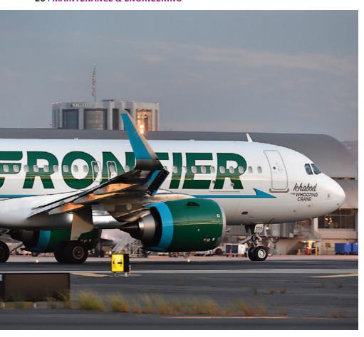
The LEAP-1A's bypass ratio of 11.0:1 is helping the A320neo achieve fuel burn reductions of 15% or more compared the previous generation A320ceo equipped with the CFM56-5B series.
