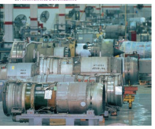
The JT8D-200 is mature engine and has short onwing times compared to modern types. The JT8D-200, however, has a lower requirement for man-hours and cheaper parts and LLPs than modern types. These counter its shorter shop visit intervals and its costs per engine flight hour are similar to modern engine types.
