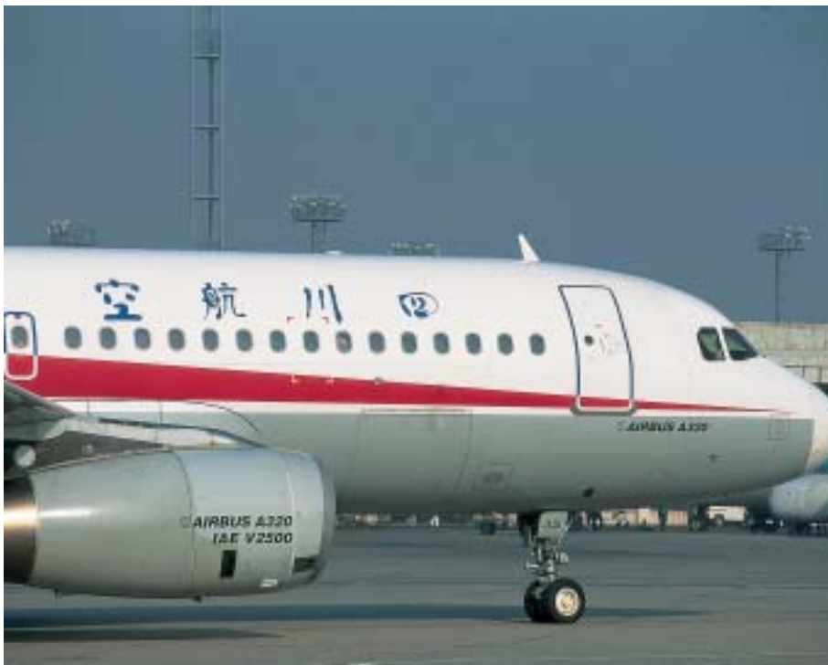
There are five variants of the V2500-A5, rated between 23,000lbs and 33,000lbs thrust. All models have uniform LLP lives of 20,000EFC.
