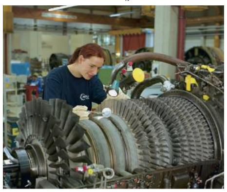
outsourced, depending on the part and the repair. Fan booster stator cases, for example, are repaired in-house, while maintenance of LPT cases requires piecepart repairs and is outsourced.
