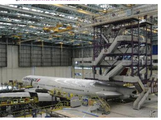
The 777 uses only about 40% of the labour per FH for base maintenance over the interval of a full base check cycle that the 747-400 consumes. The 777 has benefitted from a design that allows easier access to deeper inspections.
