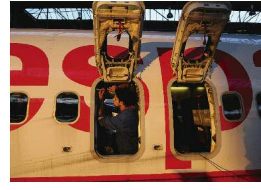
interval. According to the MPD, the actual inspections require only 4.50MH, but use several hundred MH for the removal and reinstallation to gain access.
