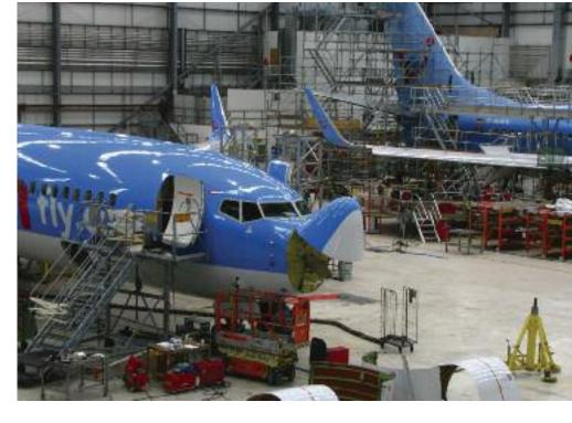
base check cycle will therefore be 21,000-22,000MH. This will be used over an actual interval of 10-11 years because of typical interval utilisations, even though the MPD interval is 12 years. This will therefore be equal to an MH consumption of 0.61-0.67MH per FH over the full cycle interval.
