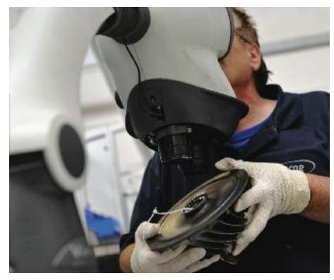
16 years, depending on part life and rate of aircraft and APU utilisation. Some will have to be replaced several times during the aircraft's operational life, while those with the longest life limits may only need to be replaced once.
