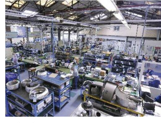
inspected as per the inspection repair manual (IRM) to a zero-time inspection. It is more difficult for a part to pass this inspection because the zero-time criteria are more stringent. Zero-time inspections involve more detailed dimensional checks, more parts require a nondestructive test (NDT), and parts are inspected using magnification of up to 10 times their size.
