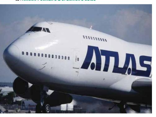
For the JT9D-7J, there is a paper modification that improves performance of the -200B when operating under Stage 3 restrictions. The upgrade is achieved by moving the centre of gravity, combined with a change in the aircraft trim. This allows a lower thrust setting to be used, resulting in lower noise levels at higher MTOW, increasing MTOW from 770,000lbs to 791,000lbs and increasing cargo capability for the -200B by an estimated 10 tons.
