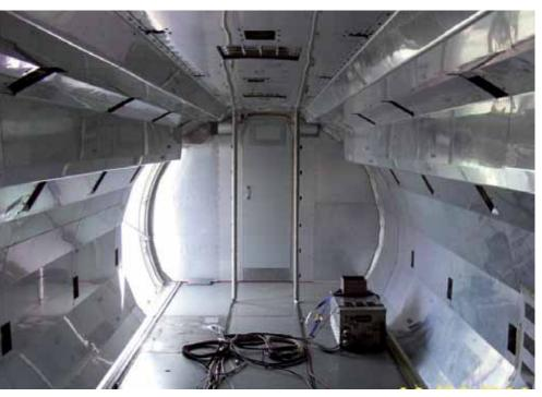
The maximum payload of the basic ATR 42 is 10,1412lbs, rising to 10,891lbs for aircraft that have incorporated SB ATR42-08-0003. In QC configuration, maximum zero fuel limited gross payload is 11,993lbs, but the cabin nets allow a maximum bulk payload of 10,582lbs and the aft cargo hold is limited to 1,693lbs, giving a maximum net bulk payload of 11,894lbs. This is reduced by 847lbs in the early aircraft with the shorter aft compartment. The maximum net containerised payload is 8,413lbs.
