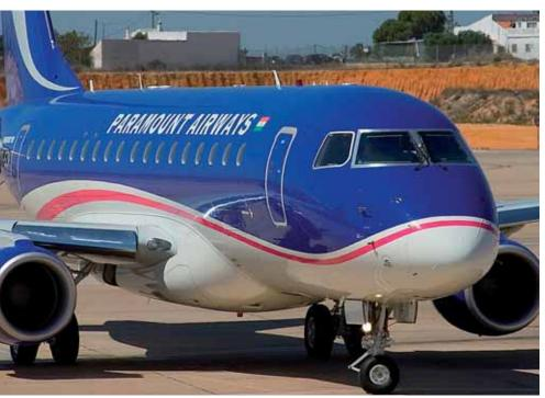
variants, is equipped with the CF34-8E rated at 14,500lbs of thrust and has a bypass ratio of 5:1.
