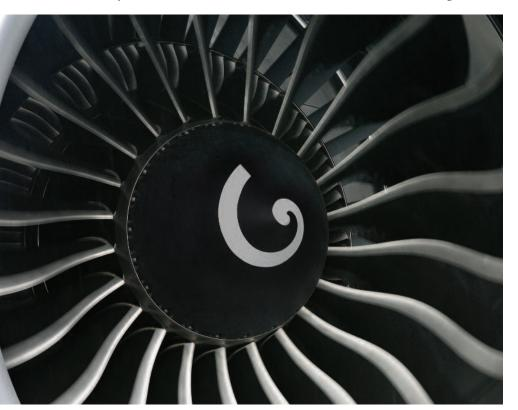
One particular technology developed for the GE90 was swept, wide-chord fan blades made with composite materials. These blades allow the wide-diameter fan to turn at a relatively high
