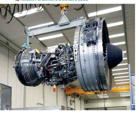
Part of the Phase III modification programme was the introduction of a new HPT stage 2 blade alloy. This was used to withstand the higher temperatures that Phase III engines run at. The unforseen problems with the new alloy, however, was internal sulphidation and external cracking. This blade material has been withdrawn and the original blade alloy is now used.
