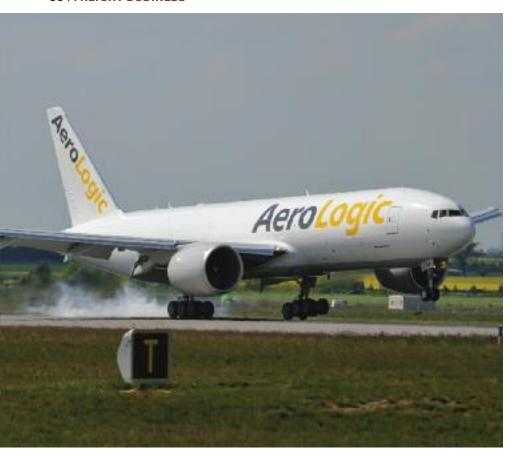
The 777F has strong operating performance, and is a consequence of its high MTOW and engine thrust. The aircraft is also in a class of its own; its structural payload falling between the MD-11F and the 747.
