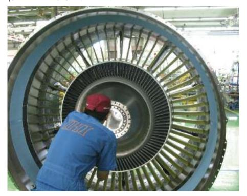
The fan and LPC modules only usually require a full level 3.0 workscope when having a full overhaul for the purpose of complete disassembly and replacement of the full shipset of LLPs.
