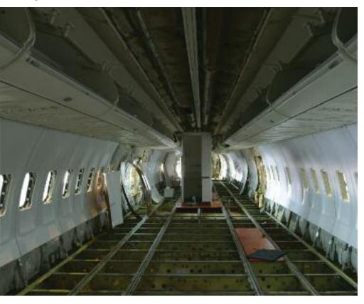
via a GVI, or an NDT, the ageing tasks aim to go beyond more than what is visible. Therefore these tasks may require sealant removals, for example, which is a step further than the requirements of the core MPD tasks." More preparation and deeper access is required for these highthreshold tasks, which will significantly affect downtime during inspections.
